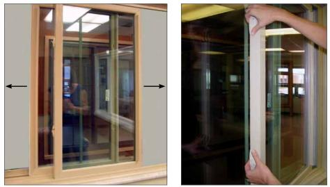
STEP 2: Open both sashes so there are equal openings at either end. On right sash, rotate cam locks to wash position and swing in like a door.
